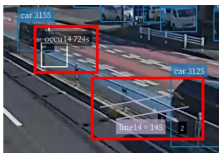
Fig.7 Measure the number of cars and occupancy time on right turn lane
